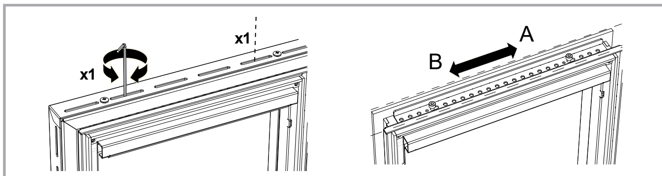
Picture 20 - Auxiliary air adjustment for glass cleaning: the plate is open at the position indicated with the letter A, while it is closed at the position indicated with the letter B.
